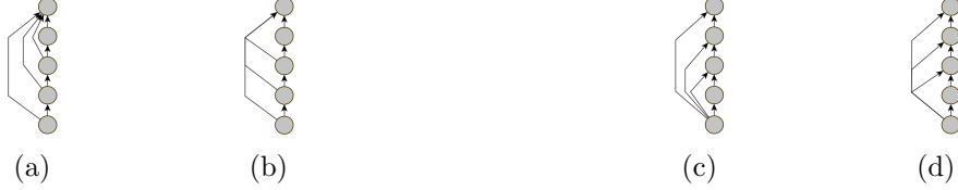
Figure 2.3: Bundling of path transitive edges: (a) incoming edges into node 13, (b) after bundling, (c) outgoing edges from node 16, (d) after bundling.
